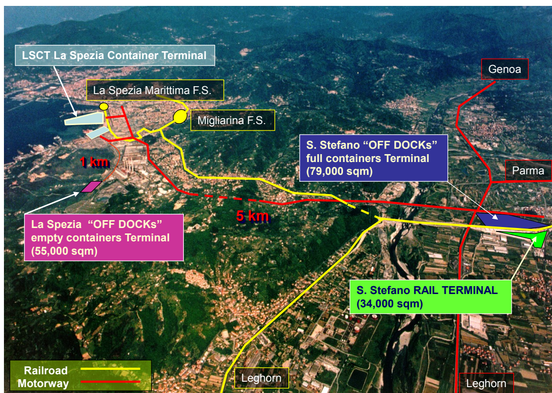
Figure 46 The off-dock system between the port of La Spezia and the “close dry port” of Santo Stefano Magra (5 km away).
