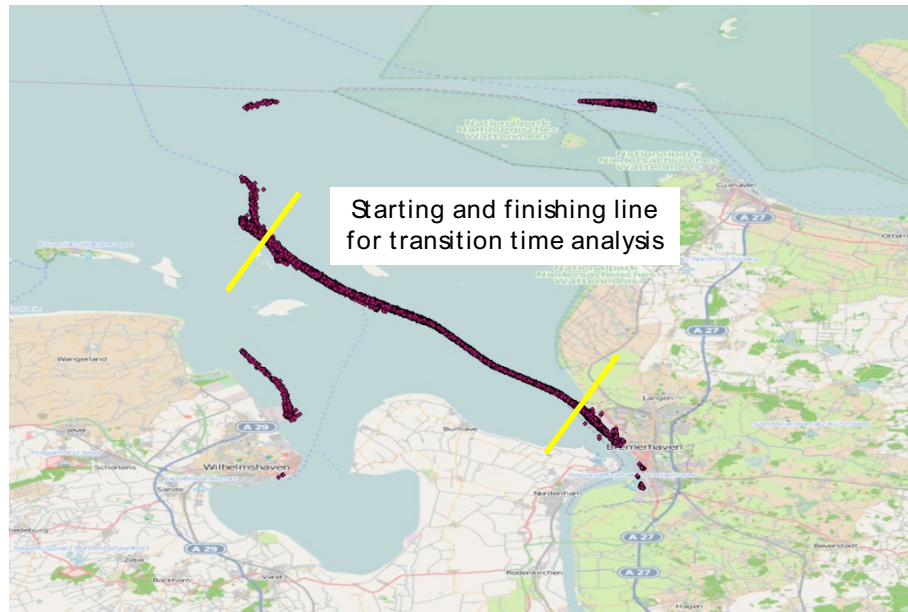
Figure 7: AIS data visualisation for the Port of Bremerhaven, ship type: container
