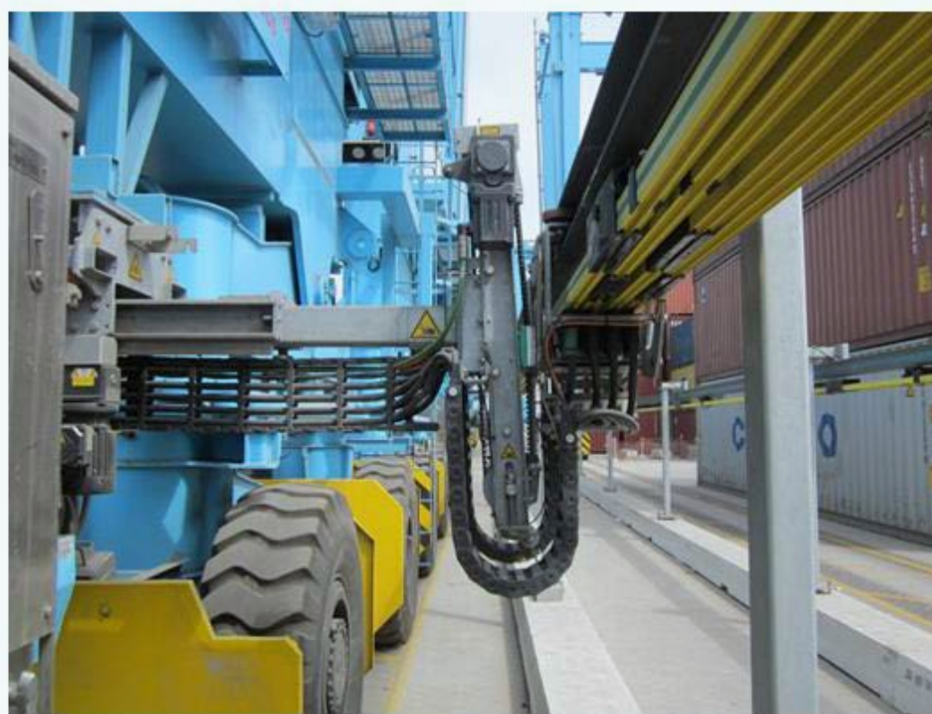
Figure: Cable reel and busbar electrification of RTG cranes (Source: Royal HaskoningDHV)
