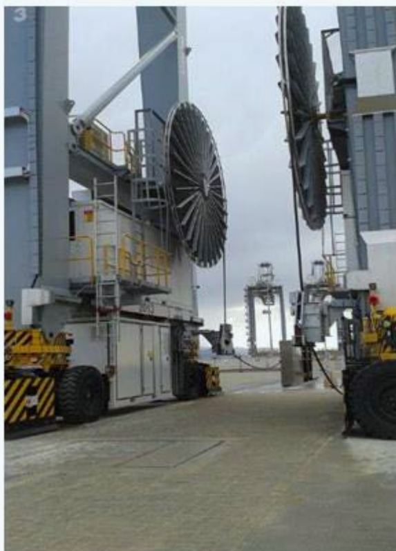
Figure: Cable reel and busbar electrification of RTG cranes (Source: Royal HaskoningDHV)
